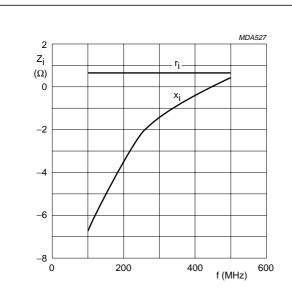
Class-B operation; V\_{DS} = 28 V; I\_{DQ} = 2 \times 80 mA; P\_L = 80 W.
