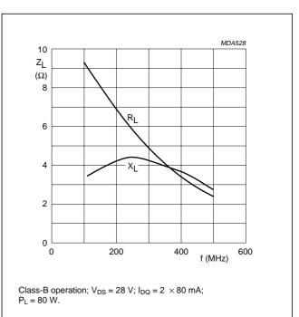
Fig.14 Load impedance as a function of frequency (series components), typical values per section.
